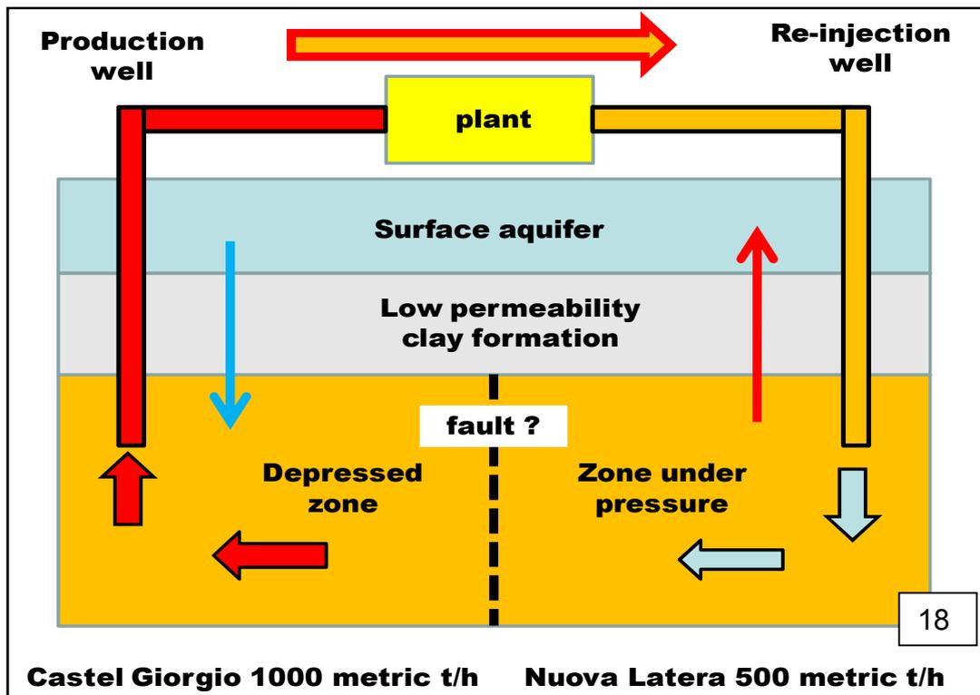
The process is based on two hypotheses: (a) the geothermal fluid can return freely from the reinjection zone to the production one: (b) the rock covering the geothermal reservoir has no permeability, thus preventing hydraulic communication between the geothermal reservoir and the surface aquifer. Both hypotheses are very questionable.
