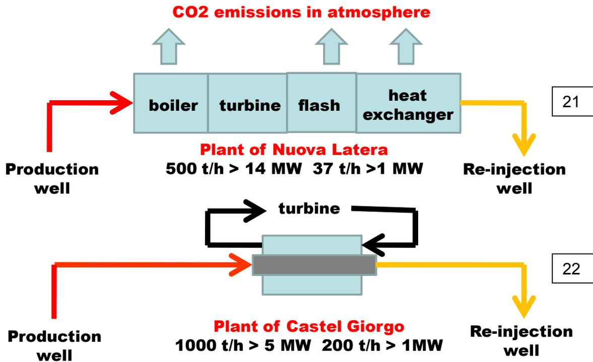
The plants called "pilot" [22] receive higher incentives because they do not emit gas into the atmosphere. The heat is subtracted from the geothermal fluid by mean of an exchanger which transfers the heat to a service fluid which activates the turbine.
